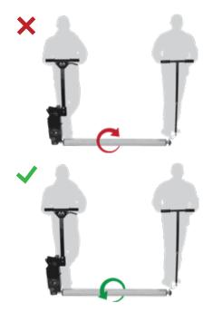
6. Once spinning direction is correct, the operator on the drive side can squeeze the speed trigger. Both operators should walk backwards in tandem to begin screeding.
