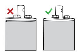
3. Equally tighten the lug bolts on the expandable pipe inserts to ensure proper fitting into pipe using a ¾" ratcheting socket, wrench, or preferrably a battery impact.
