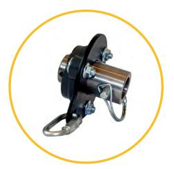
Because our drive and static pipe ends are the same, our static end attaches just like the drive chuck with one pin connect and disconnect. This feature allows the operator to change drive ends without moving the pipe.
