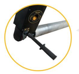
The design and placement of the heavy duty kickstand allows an operator to leave the screed free-standing during a pour without catching rebar, formwork, or falling down. Kickstand can also be removed and placed in back of handle for easy transport and storage.
