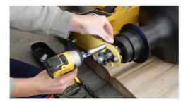
6. Lift the frame off of the drum shaft.
