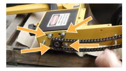
4. Remove the chain from the drum sprocket by taking apart the connector link.
