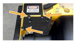
1. Remove the drum sweep assembly using the three wing nuts.
