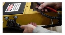
5. Unbolt both drum bearings from the frame.
